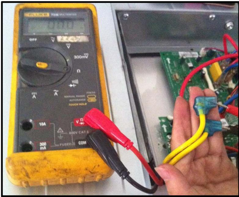
7.4.2.7 E8(Outdoor fan speed has been out of control) diagnosis and solution(Only for DC fan motor models).
